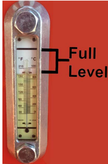
Fig. 5.1 Hydraulic Fluid Level and Temp. Gauge
