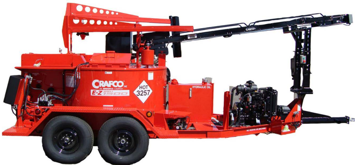
EZ1500 Series II Double Pumper Melter - Standard Hose PN 46500SB
